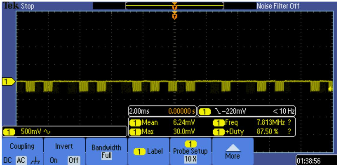
Figure 1 - Capture of IR data stream
