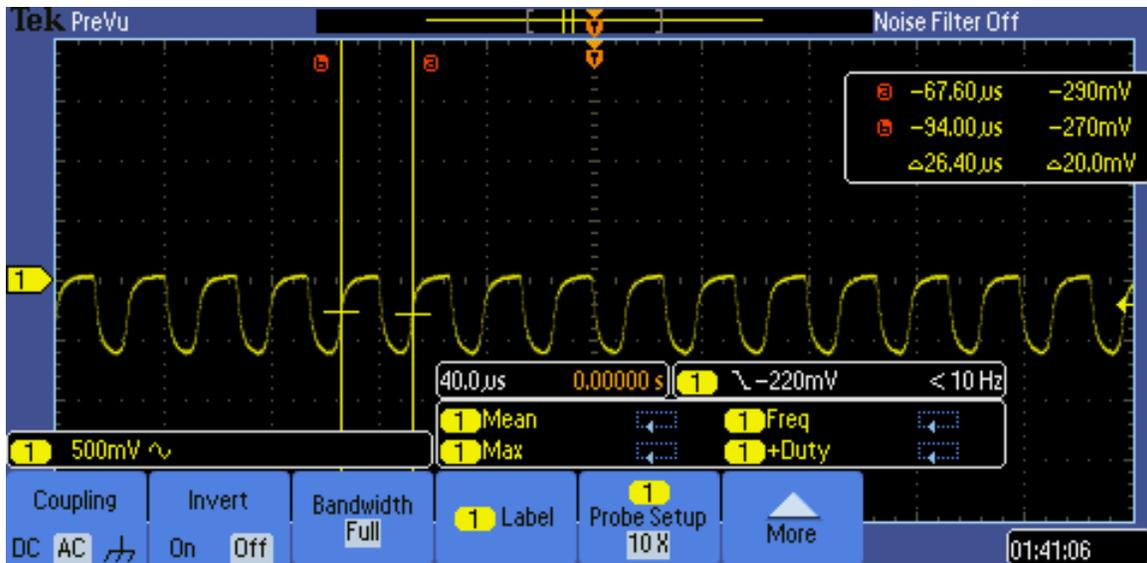
Figure 3 - Measurement of Carrier Frequency
